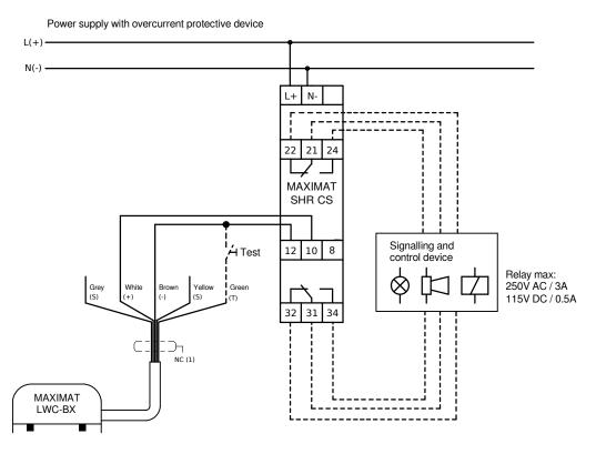
(\*) The cable shield must only be connected to a low-interference operating ground if increased EMC interference signals are to be expected.
