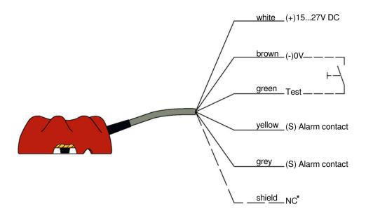
(\*) The cable shield must only be connected to a low-interference operating ground if increased EMC interference signals are to be expected.
