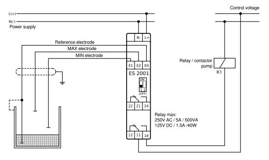
Relay of the filling pump activates when MIN-electrode becomes free; ...drops off when MAX electrode is immersed
